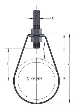
"E" dimension includes exposed rod threads beyond bottom of the hex nut. Exposed rod thread dimension is equal to the diameter of the rod used.
