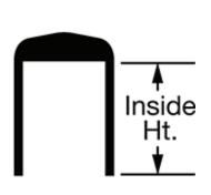
For Shape Round Cap Type Push On Flexibility Flexible Profile Straight For OD 3/8"-7/16" Inside Height 3/8" Vinyl Plastic Material Maximum 180° F Temperature
